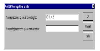
6. In the *Name of printer or print queue on that server:* field, enter the print server **output port** being used. *For example*, for port 1 enter **P1**, for port 2 enter **P2**, etc. Click **OK**.
